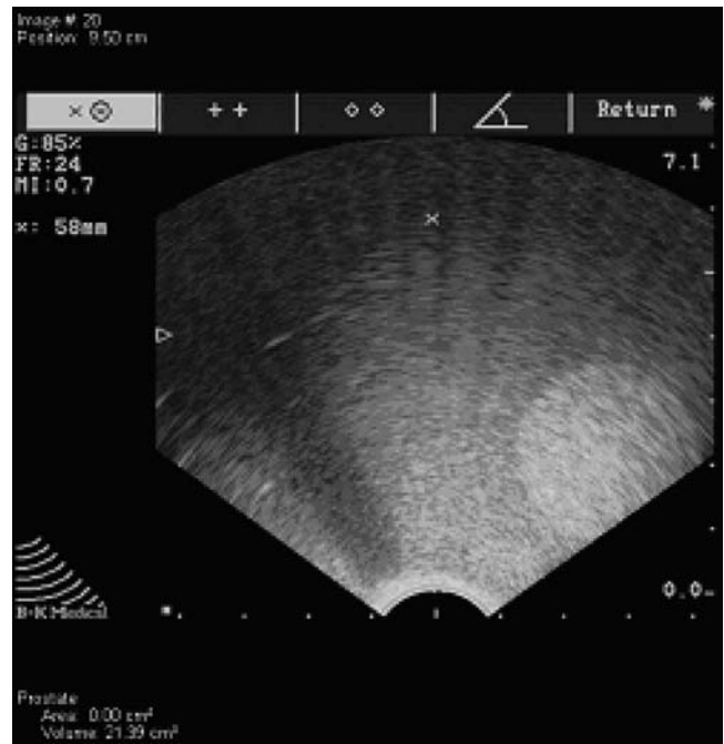
FIG. 5. Depth of penetration measurement. In this example, the maximum depth, indicated by the x (solid arrow) is approximately 6 cm (dotted arrow). The marker is located at the position where the speckle of the phantom is overcome by the electronic noise of the system.
