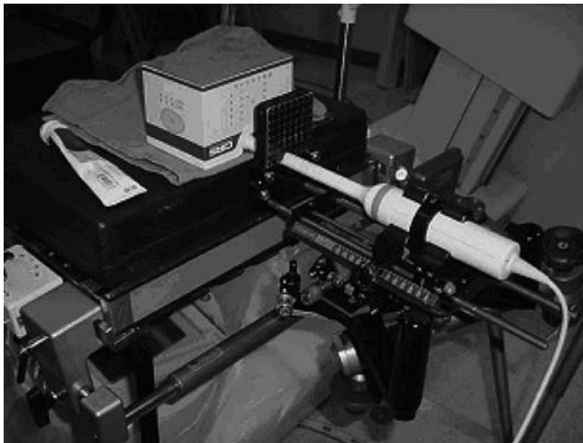
FIG. 2. Test setup. The transrectal ultrasound probe is shown passing under the needle template. Both are fixed to the stepper, which is connected to a stabilizing arm locked to the treatment table. The CIRS Brachytherapy Phantom is used in this example.
