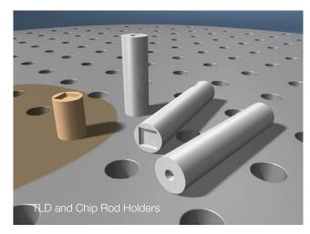
Tissue equivalent plugs cast to precisely receive TLD chips and TLD rods are an available accessory. These rods are available in soft tissue, lung and bone formulations and can also be cut to length by the end-user in order to position the TLD at the appropriate depth within the section.
