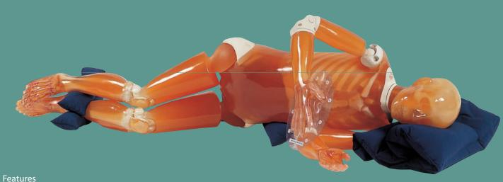
The Whole body phantom PBU-50 is a life-size, full body anthropomorphic phantom with a state-of-the-art synthetic skeleton, lungs, liver, mediastinum and kidneys embedded in KYOTOKAGAKU original soft tissue substitute. Movable joints allow basic positioning for plain X-ray and training/research applications can be enriched by disassembling the phantom into 10 individual parts (head, limbs and trunk). There are no metal parts or liquid
