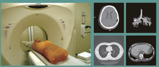
Features A one-piece anthropomorphic torso phantom with anatomical structures allows various CT approaches including helical scanning. Along with state-of-the-art synthetic bones, brain with cerebral ventricles, eye balls, lungs with three-dimensional pulmonary vessels, trachea, liver with portal and hepatic veins, kidneys, gallbladder, pancreas, spleen, aorta, cava, ureter, urinary bladder, prostate, rectum, sigmoid colon are embedded.
